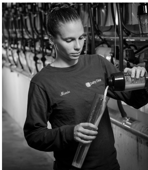
Dairy One DHIA Technician Marie Rohde takes a milk sample from an electronic meter.
